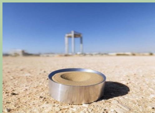
Currently, the process is costly since it requires thermal energy storage (TES) materials as well as a solar absorber, let alone their transportation to the solar plants, usually located in the world's deserts. But the UAE sand could work as both.
