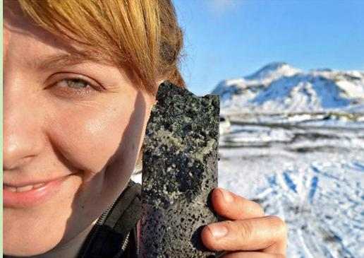
sought to solidify the CO<sub>2</sub>. Lab experiments showed that, unlike the sedimentary rocks that most other projects have used for injection, the local basalt contains plenty of calcium, iron and magnesium, which are needed to precipitate out carbon. Experiments showed that large amounts of water would also have to be added to make the reaction go-another departure from previous projects, which have just pumped down pure CO<sub>2</sub>.
