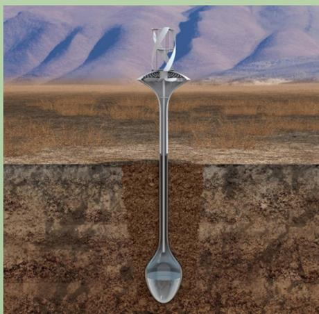
the temperature differences. It is planted six feet below the ground surface, and soil is then packed around its metal neck. The top of the Water Seer holds a vertical wind turbine, which spins internal fan blades to draw air into the subterranean chamber. Because the underground chamber of the Water Seer is cooled by the surrounding
