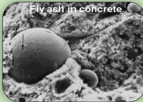
come a significant waste management issue in the world. More than 50% of fly ash ends up in landfills, where it can easily leach into the nearby environment. While some researchers have used fly ash in concrete, they haven't been able to eliminate the intense heating methods that are traditionally needed to make a strong material and thus this production does not require heating or any use of the cement.
