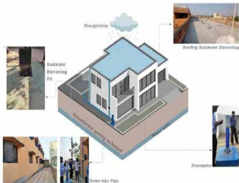
Schematic Representation of the system installed in the schools
