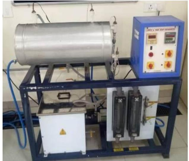
**Shell & Tube Heat exchanger**
