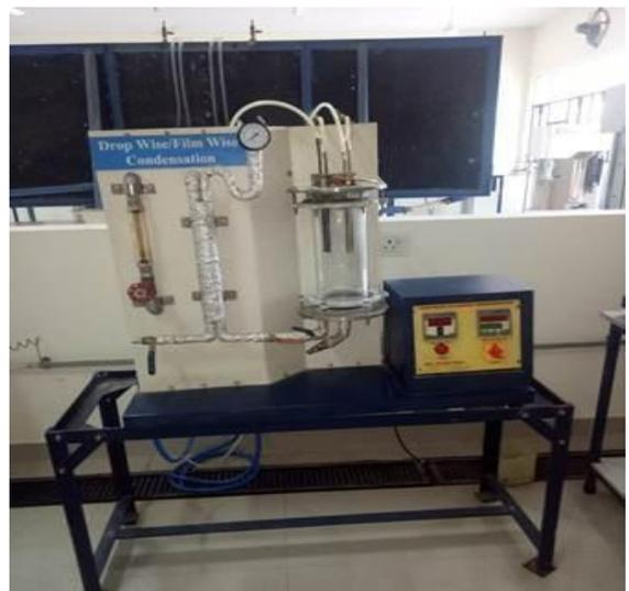
**Film and Drop wise condensation apparatus**
