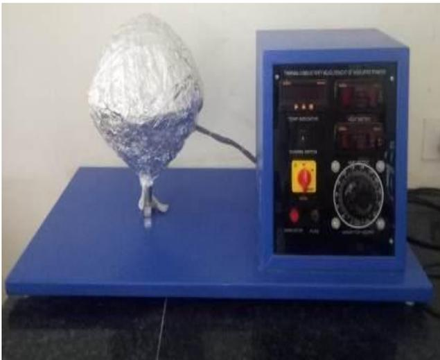
**Thermal conductivity of an insulating powder material**
