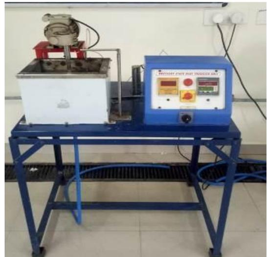
**Unsteady state heat transfer by lumped capacitance**
