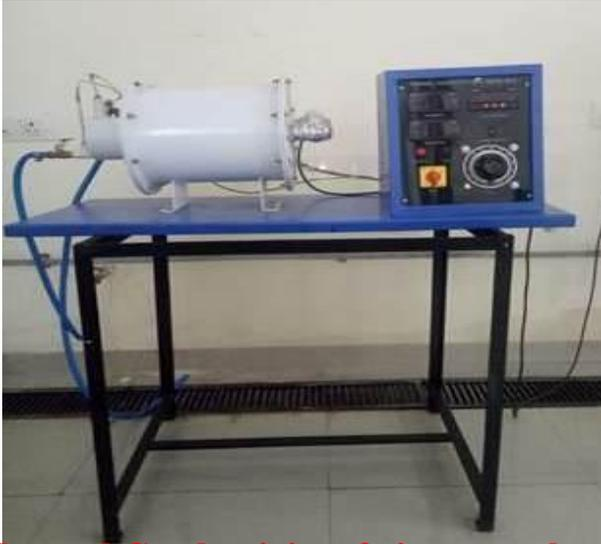
**Thermal Conductivity of given metal rod**
