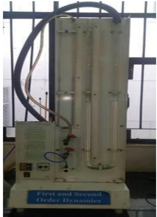
**Second order system (water-mercury manometer)**
