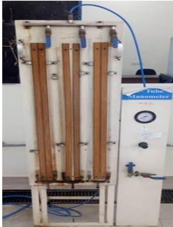
**U tube manometer three different fluids**
