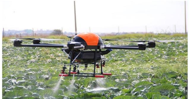
An agricultural drone is an unmanned aerial vehicle applied to farming in order to help increase crop production and monitor crop growth. Sensors and digital imaging capabilities can give farmers a richer picture of their fields. This information may prove useful in improving crop yields and farm efficiency.
